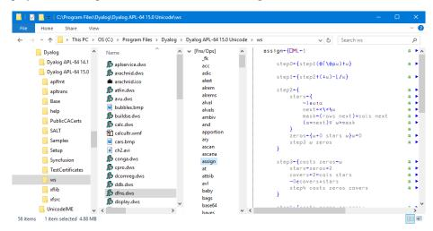
If you open the Fns/Ops node and click on a function name, the function is displayed. The next picture shows the function **assign**.
